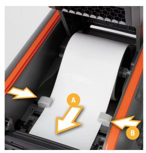
5. Feed the end of the label stock forward to reach over the roller (A). Slide the movable gray guides together so they hold the label stock neatly centered in the printer (B), without bending or wrinkling the label stock.
