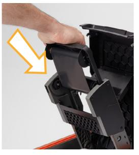
2. Slide the ribbon cartridge into the slot in the rails. The cartridge will only fit the correct way, and a magnet will hold it in place. To remove a ribbon cartridge, simply pull it out.
