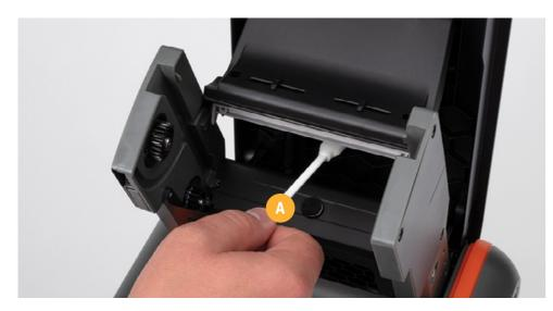
5. Lift two black latches on either side of the platen roller (C), and lift out(D)\*. Use the swab or cloth with isopropyl alcohol to gently wipe away any material that has stuck to the roller surface. Insert
