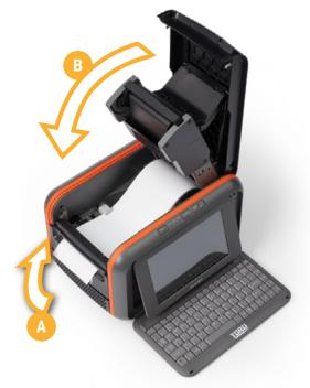
6. Lift the cutter module (A), back into its ready position; it will snap into place. Finally, lower the cover until it latches closed (B); the ribbon rails will lower into place automatically. Press firmly on both sides of lid to ensure it's properly closed.
