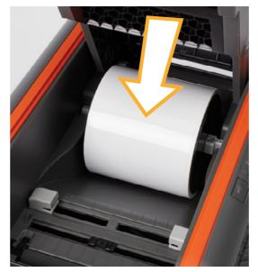
4. Place the roll of label stock onto the supply spindle\*. Rest the supply in the supply well, with the spindle fitting into its slots.
