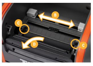
the platen roller back into printer, then press firmly down on the two black latches until they lock/snap into place.
