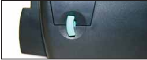
Fig. 10 Printer Release Lever being pulled forward
