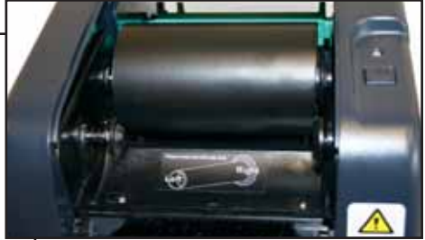
Fig. 7 Ribbon Supply (4.3") Spindle inserted at Rear Hubs
