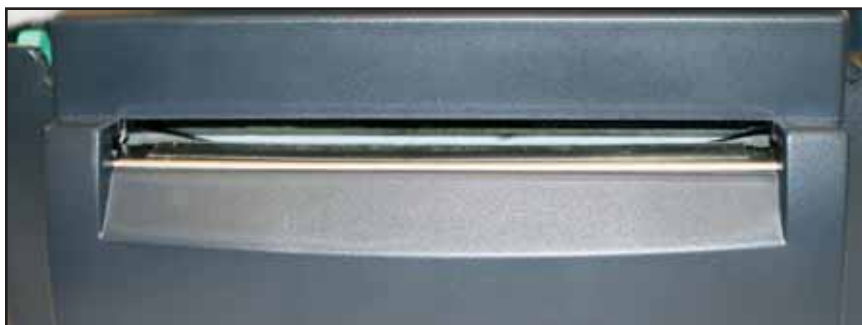
Fig. 4 Cutter (cutting blades are located at the printed label opening)
