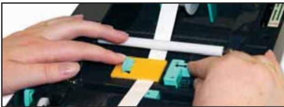
Fig. 6 Shrink tube fitted underneath and in the grooved section of the Tape Guide
