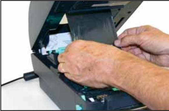
Fig. 11 Ribbon Supply (4.3") being pulled down and underneath
