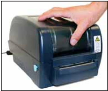
Fig. 8 Press down and in to close
