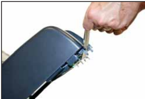
Fig. 12 Ribbon Supply being pulled up to the Ribbon Rewind Spindle
