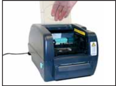
Fig. 2 Lift up and back to open
