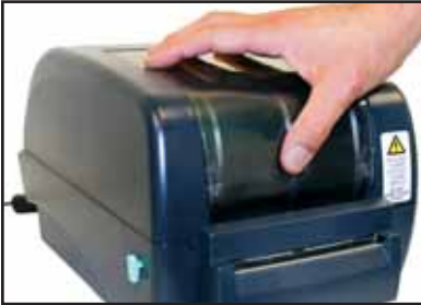
Fig. 1 Press down and in to unlatch
