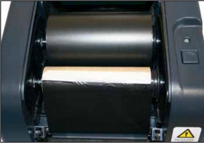
Fig. 13 Ribbon Supply (4.3") taped to Ribbon Rewind Spindle
