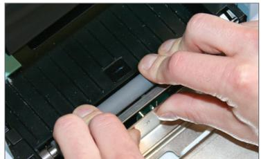
6. Run the cleaning swab back and forth several times across the platen roller. Allow alcohol to dry.
