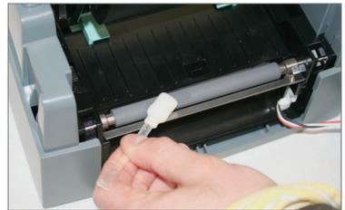
6. To clean the other side of the platen roller not currently exposed, position your fingers on the platen roller. Then, using your fingers, roll the platen roller toward you so it rotates, exposing the other side of the platen roller in need of cleaning.
