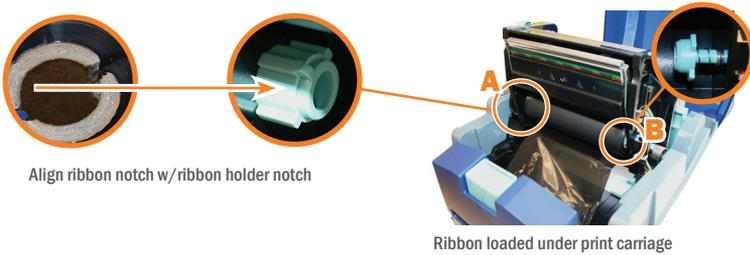
4. Extend the ribbon back over the "top" of the print carriage and, using a small piece of tape, adhere the ribbon onto the ribbon rewind core.
