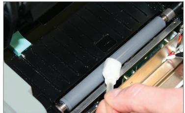
5. To clean the other area of the platen roller not currently exposed, position your thumbs on the metal plate between the electronic guillotine module and the platen roller, and position your fingers on the platen roller. Using your fingers, roll the platen roller toward you so it rotates, exposing the other area of the platen roller in need of cleaning.
