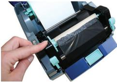
Ribbon supply taped to rewind core
