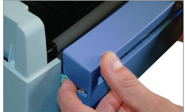
4. Open a cleaning swab, and place the swab between your index finger and your thumb. Squeeze the swab until it snaps. Alcohol will be distributed to the cotton side of the swab. Run the cleaning swab back and forth several times across the platen roller. Allow alcohol to dry.
