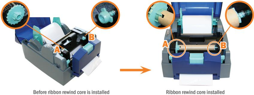
**NOTE:** Make sure to align the notch on the ribbon rewind core with the notch on ribbon rewind holder A. You may rotate the ribbon rewind wheel to help align the ribbon rewind core.
