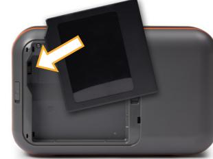
Push the battery in until it locks into place, and return the battery cover door to its position.
