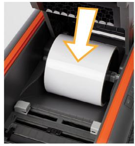
4. Place the roll of label stock onto the supply spindle\*. Rest the supply in the supply well, with the spindle fitting into its slots. Feed label stock toward the cutter module, with the printable surface facing upward.
