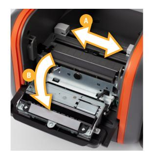
3. Slide the movable gray guides apart (A). For more room, flip the cutter module down (B) by pulling the top edge away from the body of the printer.
