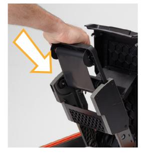
2. Slide the ink ribbon cartridge into the slot in the rails. The cartridge will only fit the correct way, and a magnet will hold it in place. To remove a ribbon cartridge, simply pull it out.
