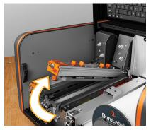
Unlatch one of the print heads and raise it by its orange tab until it can no longer be raised where it will hold.
