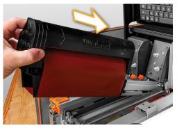
2. Holding the ribbon cartridge on the side imprinted with the DuraLabel logo (with the rolls facing up), insert it into the printer so the loose section of ribbon, on the bottom side of the ribbon cartridge, is positioned beneath the print head.
