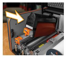
Slide the cartridge onto the rails of the print head. It should slide smoothly back until the number on the print head is visible; you may hear the cartridge click into place.
