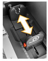
Squeeze the orange tab on the adjustable supply holder, and slide the holder to the mark for your supply's width.
