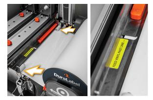
**4.** Slide the adjustable supply guides together ensuring the supply remains between the two guides and under the white rollers. Push the supply forward, under the metal guide with the orange sensor to the line shown on the yellow label.
