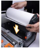
Rest the gears on the supply's end caps into the slots on the supply holders. The end cap with the DuraLabel Printers and Supplies label should face away from the inner wall of the printer.
