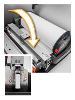
**5.** Lower and latch the feed roller in place.
