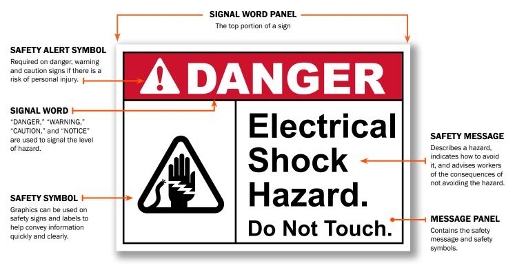
**NOTE:** Labels requiring OSHA compliance should follow OSHA and ANSI Z535 design standards to offer the highest level of safety. Be consistent in design so labels and signs are uniform. Variation may diminish recognition and add confusion to signs. Consistent design, color, safety symbol, signal word, and signal word panel are critical.
